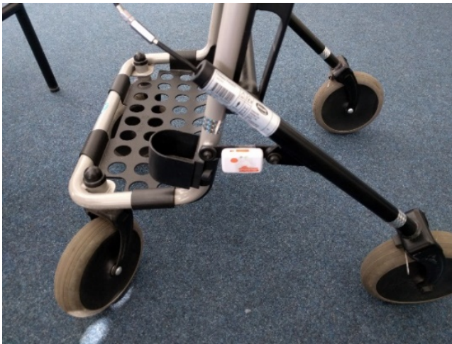
Figure 3. Displaying the apparatus; a rollator attached with a Shimmer3 IMU.
