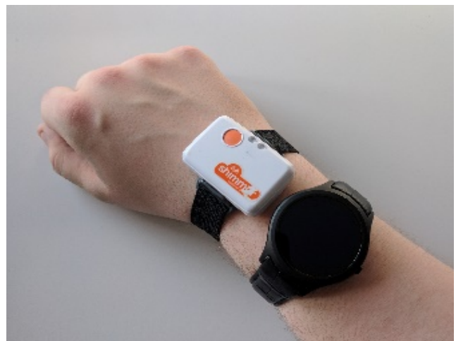
Figure 4. Shimmer3 IMU and an Android No.1 D5+ is worn at the wrist.
