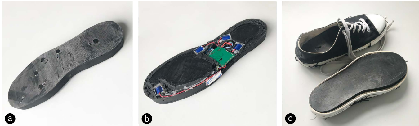
Figure 2: We further developed the prototype PNEUSHOE [12]. (a) Top view of the insole showing the mounted coin-cell vibration motors. (b) Bottom view of the insole, illustrating the pneumatic valves (in blue) and the printed circuit board (in green) housing all electronics and the integrated battery. (c) The insole placed within a modified shoe, replacing the original sole to form the complete footwear prototype.
