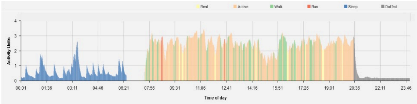
Figure 6. Typical 24h-Activity diagram with sleep (blue), charging period (gap), activity period (green and orange) and doffed state (grey).
