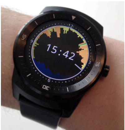
Figure 3. Radial visualization of standard activities over the day (Implemented on an LG G Watch R)
