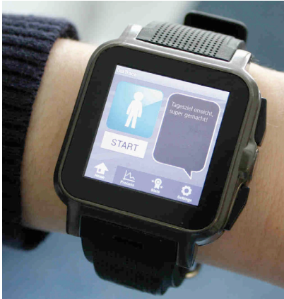
Figure 2. Detection of muscle tremor and current activity state. (Implemented on Simvalley AW-420.RX)
