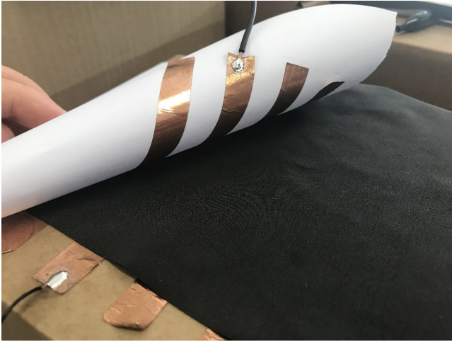
Figure 4: Showing resistive Sensing setup for copper electrodes. A black velostat material is the buffer layer that is permeable and changes the conductivity at pressure.
