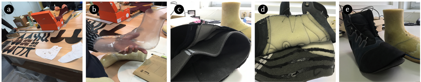
Figure 1: The process of building a 3D foot scanning shoe begins with preparing materials and design templates (a) and progresses to creating a transparent mold (b) for precise shaping. The inner lining (c) is integrated with conductive elements, ensuring both comfort and functionality. Conductive ink electrodes are then embedded onto the shoe's lining in specific patterns (d) to enable advanced sensing capabilities. Finally, the fully assembled shoe (e) combines ergonomic design with innovative sensing technology, resulting in a wearable prototype.
