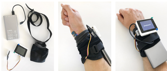
Figure 1: Left is showing the components, which are a wired gas sensor break-out board, Wio Terminal, 10,000mAh VARTA powerbank, Velcro strips, sock, and a USB cable. The middle photo shows the sensor mounting at the wrist. Right image shows the screen displaying the classified substance.
