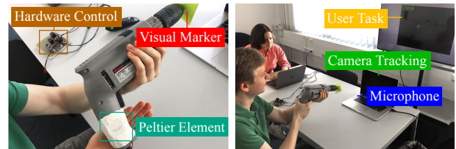
Figure 3. A peltier element (TES1-127025) is attached to the handle of a drill. In a lab environment, the subject had to aim at moving circles displayed at a 50" screen and drill them into thin air. The position tracking is done with an RGB webcam and drilling is detected by the microphone.
