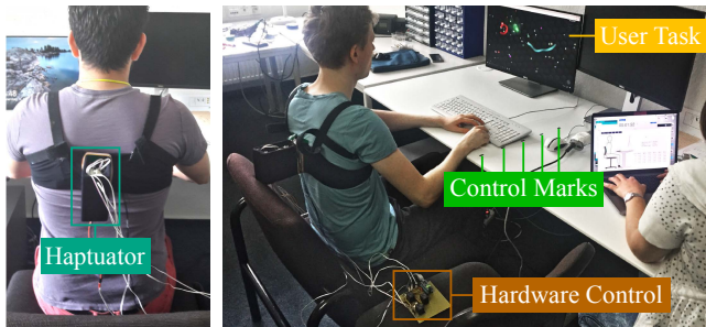
Figure 2. The haptuator is tightly mounted to the user's back using velcro tape. The user is playing Slither.io, while the study leader triggers random notifications. The back's degree-angle, calculated from an accelerometer, is being constantly logged. Also, 5 different keyboard distances were tested.
