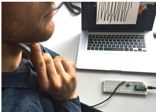
Figure 2. Pressing the pen against the throat, enables a sensing of micro-eruptions caused by the pulsing blood. An Arduino Nano (ATMEL Mega 328PU) is used to push the data stream through a Serial connection, in order to visualize date on a computer in real time. A future product would also display the data at the pen and push the data on a server.
