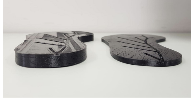
Figure 8: Image of the 10mm and 5mm insoles 3D printed from flexible filament (Ninjaflex [39]).
