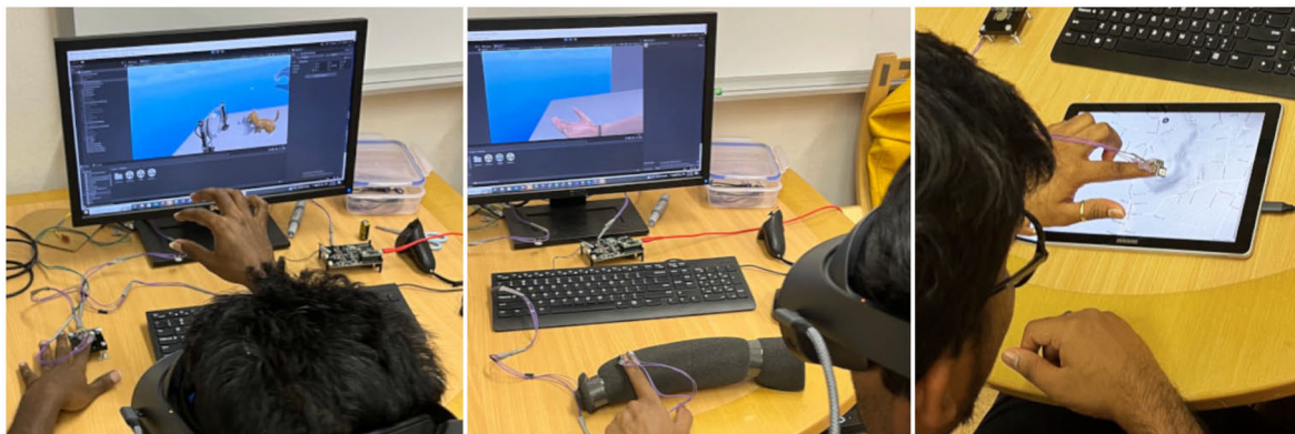
Figure 9. A virtual cat is walking from right to left and the user can feel it touching their index finger with its head (left). The user can feel the pulse of a virtual arm the closer they get to the wrist (center). The user can feel the elevation on a 2D map (right).
