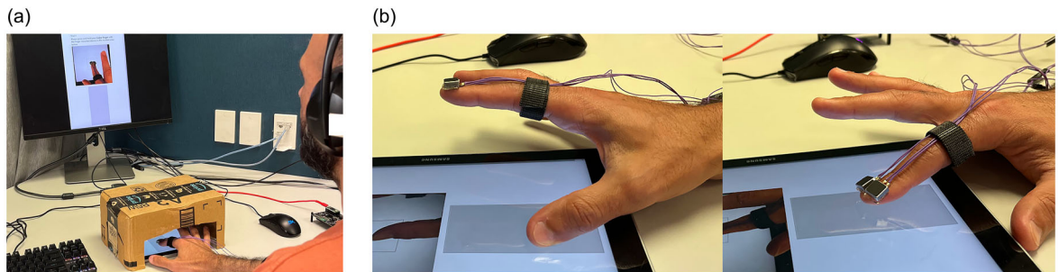
Figure 3. (a) Setup and Apparatus. (b) Two conditions. Study 1: (a) a cardboard box acted as a visual barrier to prevent the user from observing the LRAs. (b) There are two different INTERACTION_SPACE conditions: (1) IN-AIR : the participant touches the screen surface with the thumb while lifting the index finger up. (2) ON-SURFACE : the participant touches the screen surface with the index finger directly.
