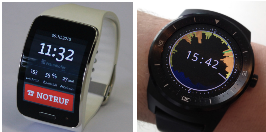
Fig. 1. Prototype of the DHC system implemented on a Samsung Gear S Smartwatch (left) and Activity watchface implemented on an Android Wear LG G Round (right)
