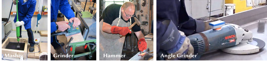
Fig. 1. Typical tools that are used in a various kinds of shop floors may include a masher, grinder, hammer, angle grinder, and many more. All these tools emit considerable hand-arm vibration when used, which is unhealthy and should be tracked by the worker as demanded by legal regulations in European countries such as Germany.
