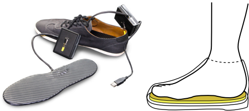
Figure 3. The insole can be inserted in any ordinary shoe and can be connected via USB or wirelessly via Bluetooth.
